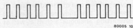
Figure 10. The IC transmits the five-bit code in a chain of six pulses (two of the pulse trains are shown). The information is contained in the interval between pulses: a logic 1 gives a short pulse, logic 0 is coded as a longer interval. Both pulse trains shown here give the same code: 10100.
